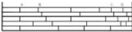
Above, recommended layout of flooring. End joints should be spaced between 15-18" apart.
